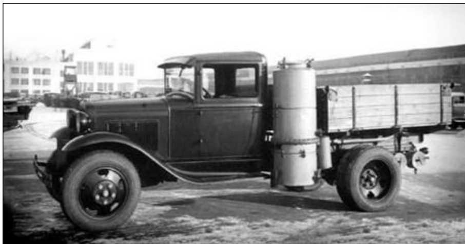
A Soviet GAZ-14 truck (Ford AA truck) with a gas producer (Aussie A Models Facebook page)
