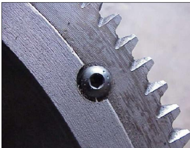
The setscrews lock the ring gear to the flywheel
