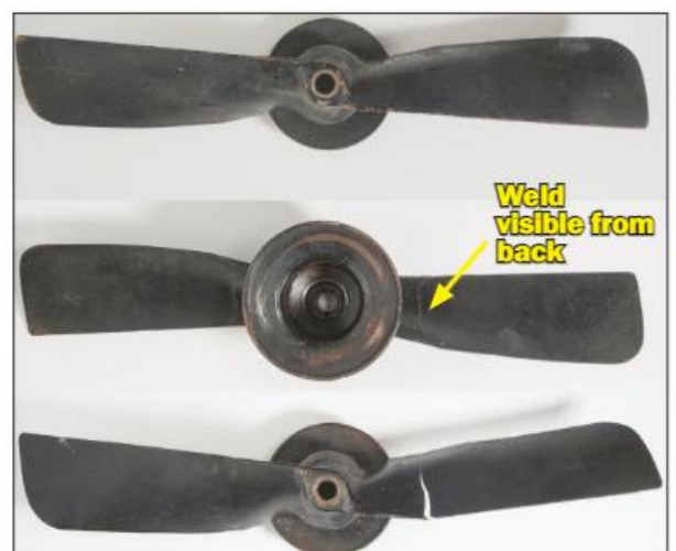
Figure 4. Failed Holley fan.
