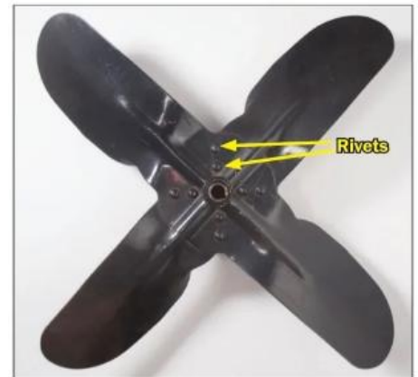
Figure 5. Original 1933 four-bladed fan.
