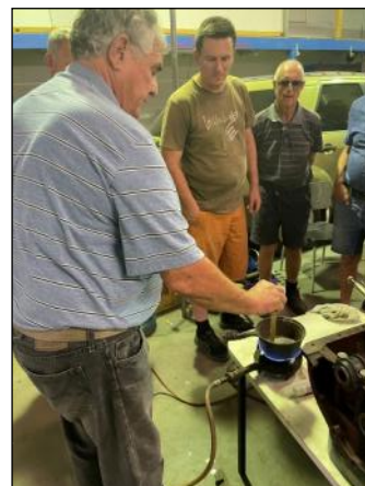
Step 4. Steve Read using the official Ford method to test whether the white metal is at the right temperature (must just char a piece of pine wood)
