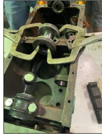
Step 2. Babbitt mould clamped into position
