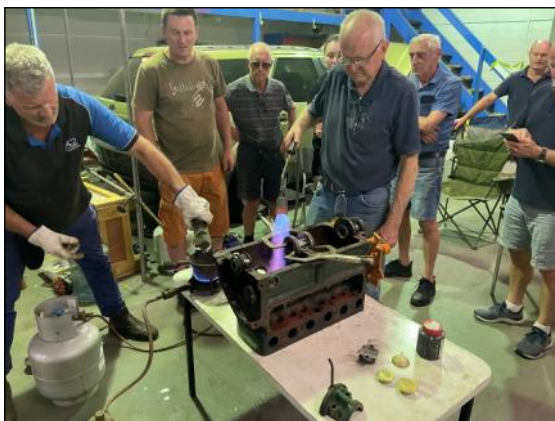
Step 3. Ray Major melts the new white metal while Ron Andrews warms the block and mould.
