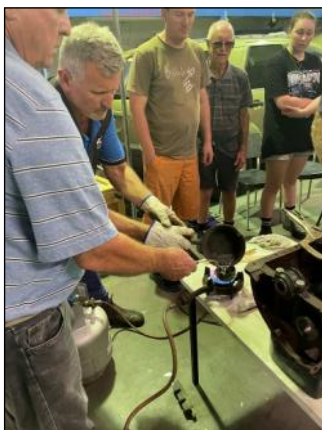
Step 5: Molten white metal is transferred to a ladle
