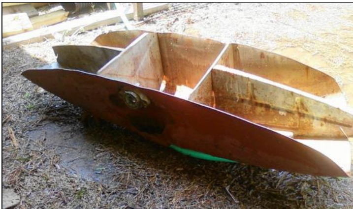
Inside a Model A fuel tank
