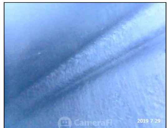
Nice even distribution of the internal sealer
