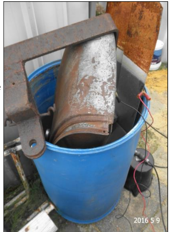
Electrolytic de-rusting in process
