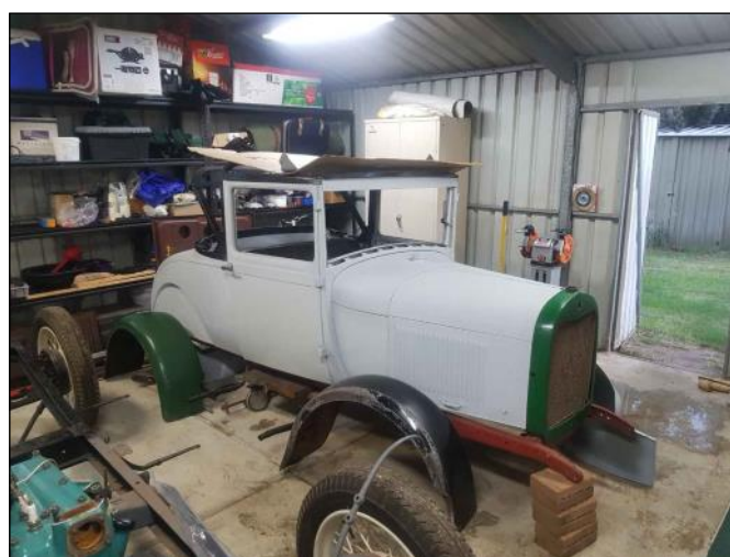
The new body waiting to be mated to the (partly visible) chassis
