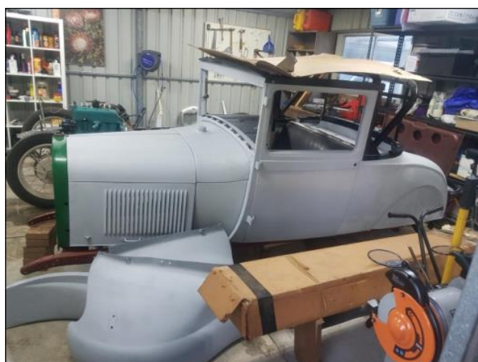
The new body waiting to be mated to the (partly visible) chassis
