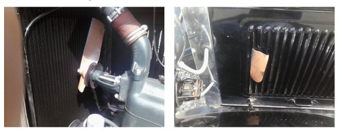
The original four blade fan can also be a disaster. It has two separate metal blades which have four steel rivets holding it together. The problem here is that over the years the vibration has cracked one or several of these rivets and it is only a matter of time before they let go and the two blades fly around inside the closed bonnet doing lots of damage.
