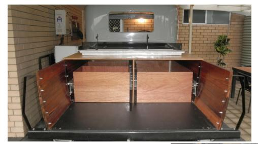
The sides are made from jarrah floor boards, thanks to Ian Paisley! My floor and large drawers from marine half inch ply. The two drawers are 900 long, 450 wide and 300 deep. 42 skateboard sealed roller bearings ensure a drawer will slide out past the end of the tray. This is necessary because half the floor space has a deck to store the bedding.
